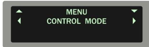
To access the DAS-8001 control modes selection menu, press the menu key and the first menu option of **CONTROL MODES** appears on the display. Press the down arrow and the following options on the line below may be scrolled through using the right and left arrows: **NORMAL, BYPASS, KEYBOARD CONTROL, CODE SWITCH**. The unit will prompt you to **ENTER TO SAVE** which will then automatically exit you out of the menu and to the **READY** screen.
