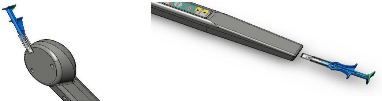
You will notice that when the transponder is in the needle, it must be held very close to the probe. This is because the metal in the needle reduces the read distance. Reading in the needle is best done by touching it to the tip of the probe, in line and 90% down.
