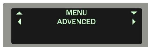
Whereas the command and setup menu divide their functionality between a one-time action item and a persistent state, the advanced user menu contains both. The advanced user menu contains functions that can be very useful, such as the function that returns the unit to factory defaults.
