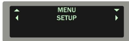
These options all have in common that they set a state in the DAS-8001 that is persistent. Simply make your selection by using the left arrow and right arrow, and then the down arrow to move down further into the menu and your left and right arrows again to make your final selection. The unit will prompt you to **ENTER TO SAVE**. Use your up arrow key to move back up into the previous menu or to move on to your next item. You can simply use the up arrow to fully exit out once you are done.
