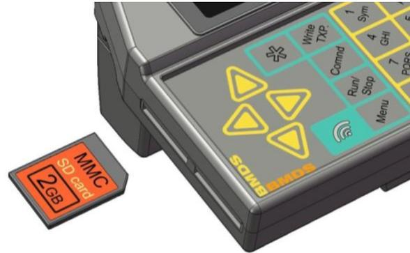
Map and Data files can also be made directly on the DAS-8001. This is done under the Commands menu. After collecting data internally you can send data to a card. If the card is formatted, the DAS-8001 will go ahead and make a data file (.txt) using the date as a file name. It will make a new file each time this is done (though no more than once a minute). See section 13.3
